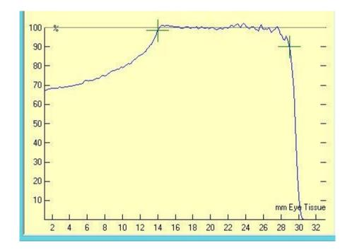
The QEye measures depth doses, using a multi-leaf Faraday Cup consisting of 512 copper sensors, spaced with insulating films. Designed to measure the entire energy range required for ocular treatments
