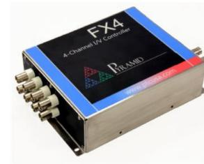
Four channel precision electrometer, applications include
