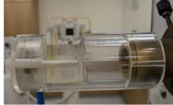
Advanced Markus chamber in a jig on the end of the beam line
